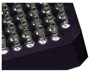
Figure 6. Micro-Coil Springs attached to CCGA.
