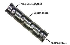
**Figure 3.** Pb80/Sn20 copper wrapped solder column without fillet (shown after coating with Sn63/Pb37)
