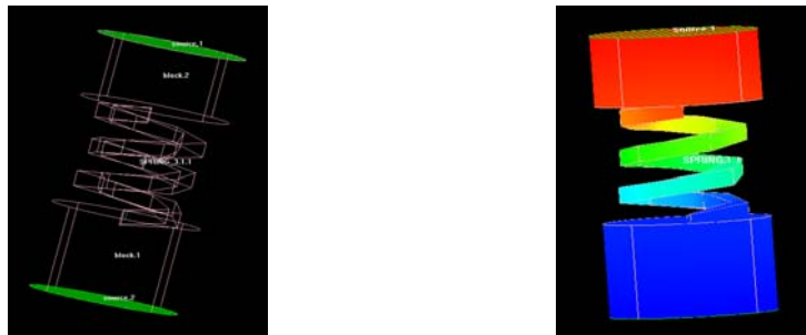
Figure 1. Thermal Simulation and Geometry of Micro-spring. Left: The wireframe of the completed geometry before the simulation begins is shown. Right: Using IcePak, it is possible to see the temperature gradient through the micro-spring.
